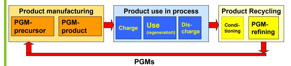
E.g. Oil-refining catalysts, chemical catalysts, glass-equipment
